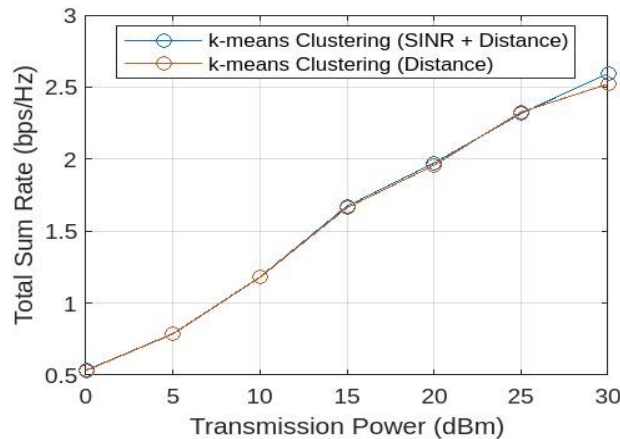
Figure 5 Comparison between the overall sum rate of k-means (SINR + Distance ) and k-means (Distance only) when 500 users are clustered
